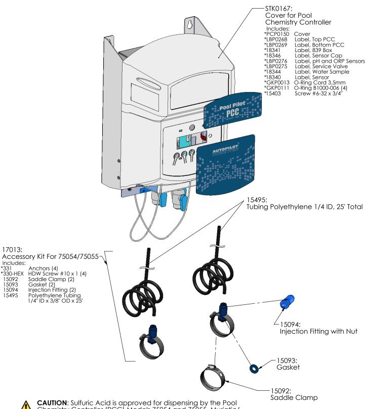
**CAUTION**: Sulfuric Acid is approved for dispensing by the Pool Chemistry Controller (PCC) Models 75054 and 75055. Muriatic/Hydrochloric Acid is **NOT** approved for dispensing by the PCC and will void warranty coverage if dispensed by the PCC.
