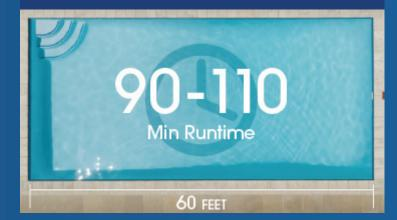
Click, drop, and let AquaClean take charge. Equipped with a best-in-class 8800mAh rechargeable battery, revel in up to 110 minutes of continuous cleaning for pools up to 60 feet. Plus, its rapid charging capability delivers a fully charged unit in just 4.5 hours, ensuring uninterrupted cleaning sessions.
