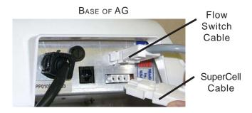
A Flow Switch Jumper has been provided with your AG system to disable the water flow switch when used with the 75093 and 75092 manifold
